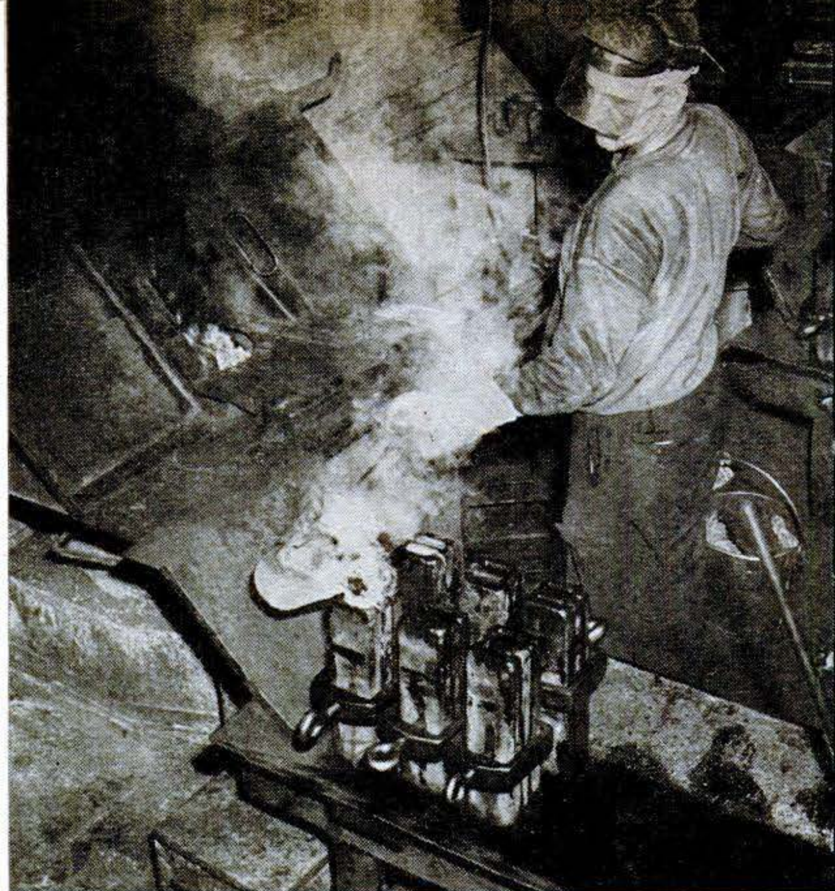
1. From a glowing crucible, a mint worker dips alloy and pours it into molds. When cool, the metal will be in the form of "coinage ingots" 12 inches long, two inches wide, and one-half inch thick. The alloy consists of nine parts silver to one part copper—the copper makes the coins tougher. Each ingot must meet rigid assay tests for purity.
